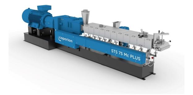
The new Coperion STS 75 Mc PLUS twin screw extruder achieves up to 20% greater throughput with improved product quality, at an increased specific torque of 13.6 Nm/cm<sup>3</sup>. *Photo: Coperion, Stuttgart Germany*
