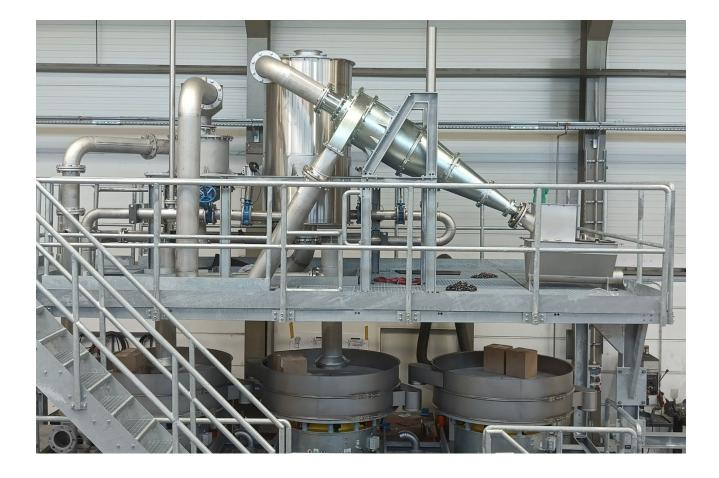
**Figure 3:** Like the entire PET recycling plant, the hydrocyclone stage for Doğa is designed for an output of 100 metric tons per day.
