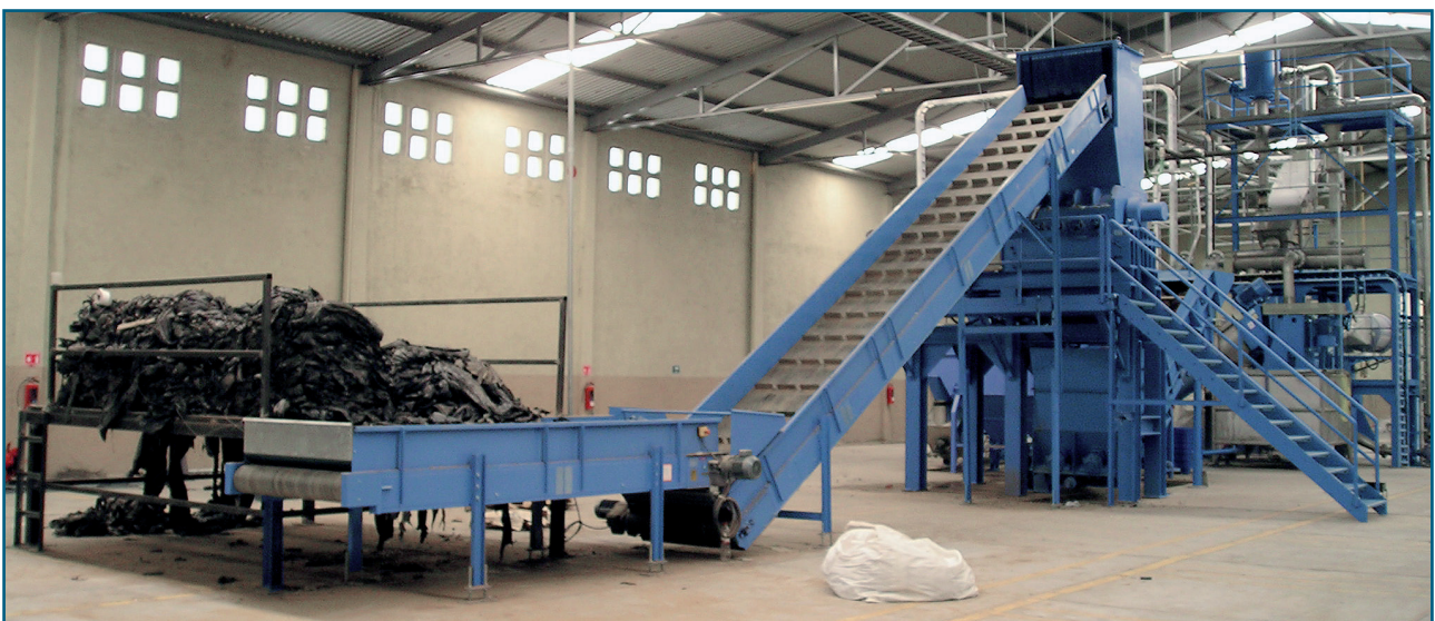
Fig. 3: Abovefloor belt conveyor with sorting table for separating the materials
