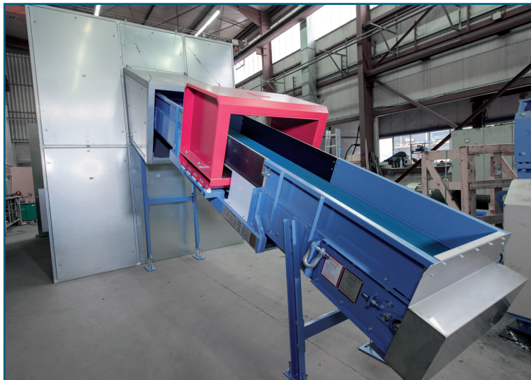
Fig. 5: Conveyor belt with metal detector and sound insulation cabin
