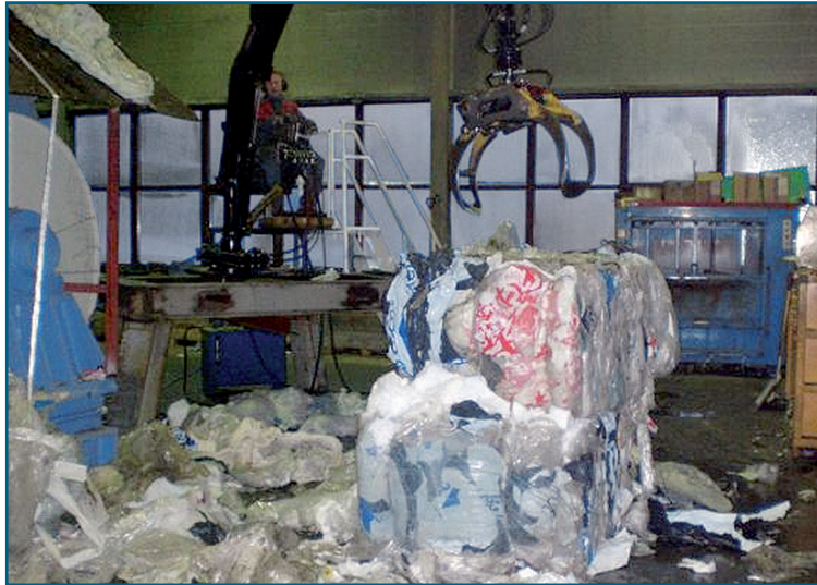
Fig. 4: Direct feeding into the size reduction machine
