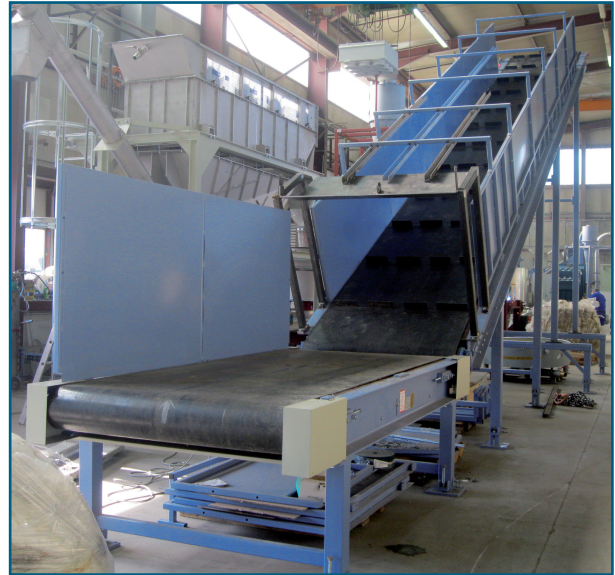
Fig. 1: Abovefloor belt conveyor for entire bales with feeding belt, manual removal of binding wires
