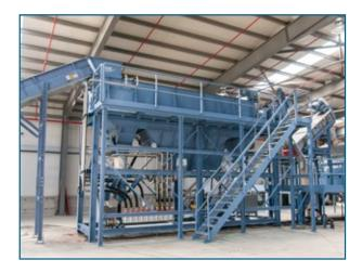
In comparison to the dry processing, the wear and maintenance costs of all three processing steps of a washing line will considerably be reduced. The washing line itself is no longer strained by heavy contaminations, the components have a longer life time and also the final product quality will improve. The water treatment has to cope with less contamination thanks to the separate circuit that can be installed in the VWE unit.
