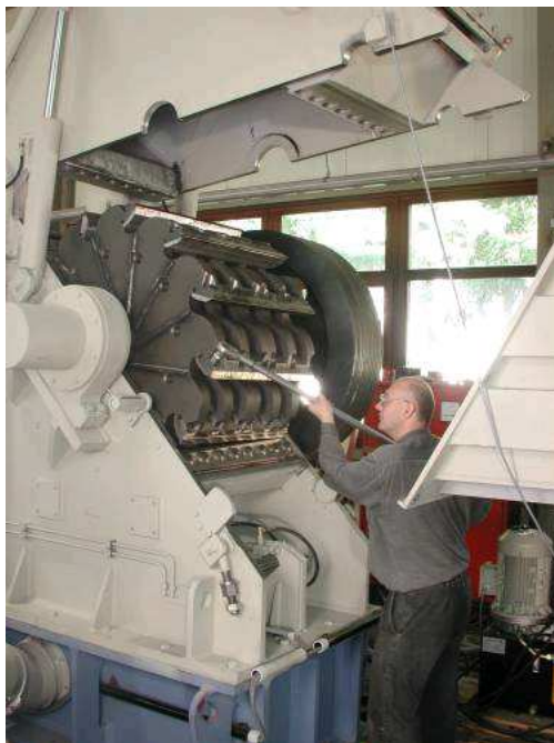
Rotor blade fastening by means of a torque wrench on a HERBOLD pipe granulator, type SMR 80/120
