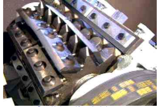
Rotor blades and fastening bolts on a HERBOLD profile granulator of the SMP series
