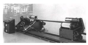
The solution: A sawing device for cutting large diameter tubes axially into long strips that can be granulated in a standard tube granulator.
