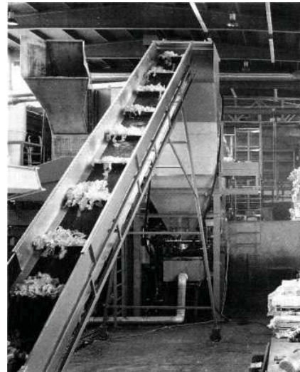
Figure 6: Granulator with a downstream swim-sink tank
