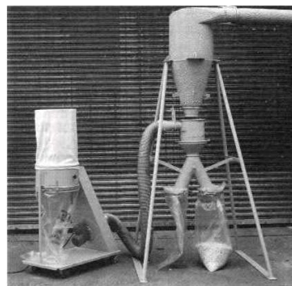
Figure 5: Suction device for granulate with dust classifier
