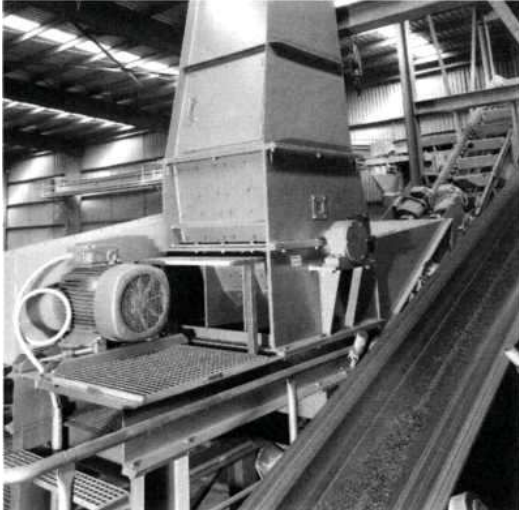
If requested we carry out the planning and the commissioning of complete systems - the photos show a down stream reduction system at a compost plant.
