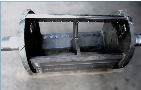
Fig. 1: The guillotine rotor without continuous rotor shaft and with scrapers between casing wall and external rotary disc.
