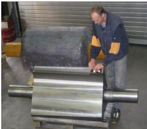
Fig. 1: Forging and machined "A" rotor
