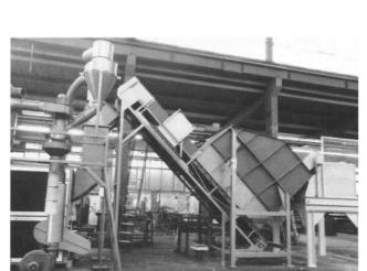
As an accessory for a central plant, we suggest the use of an automatic feed system consisting of a tipping device for containers and a dosing conveyor equipped with a metal detector. In addition, we recommend a follow-up plant such as an air separator for the separation of fines, an exhaust filter and a metal separator.
