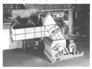
HERBOLD has developed a new type of feed device which solves these problems in a surprisingly simple manner. The material, fed in bandles is separated and fed into the granulator in portions. Thr grinding chamber is hermetically enclosed as soon as the feeding process commences.
