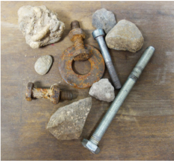
Fig.1: Example of separated heavies and extraneous material from good material PET bottles in a recycling plant.
