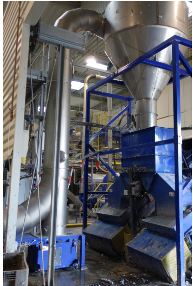
Fig.3: Ascending pipe with discharge chute and for discharging the good material in a ballistics
