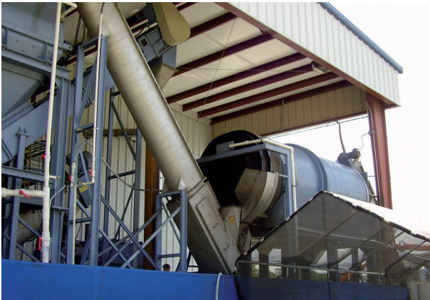
Fig. 5: Agricultural film wash drum with feeding screw
