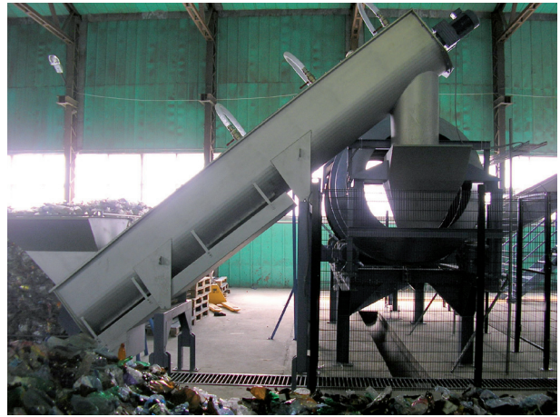
Fig. 4: PET wash drum with upstream feeding screw
