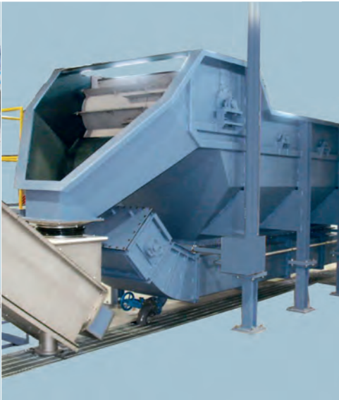
Flotation tank with scrape conveyor
