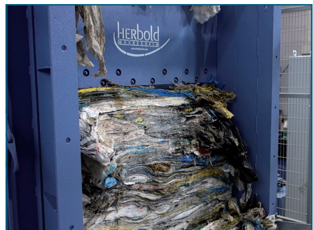
Fig. 2: Cutting the material portions lying under the cutting blade
