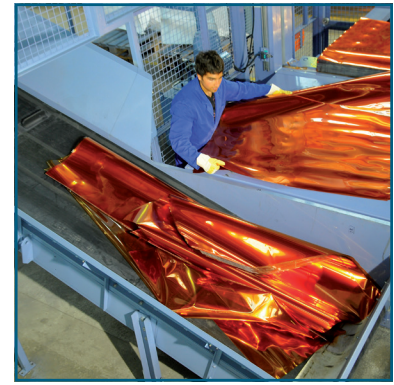
Step 3: Material portions are transferred for further shredding
