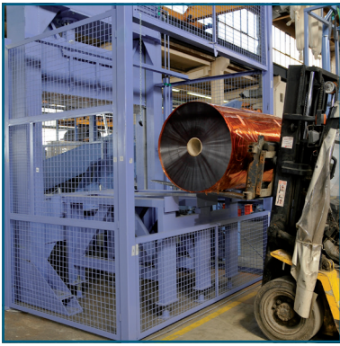
Step 1: Feed in of material is done via fork-lift truck
