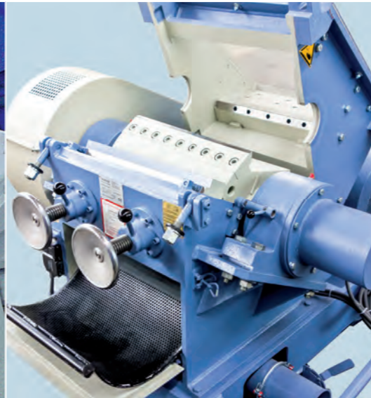
Hinge-mounted screen support of the SMS series
