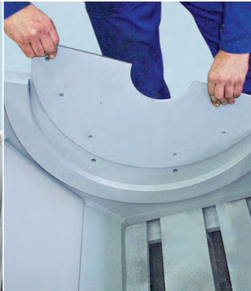
Housing with exchangeable armour plating
