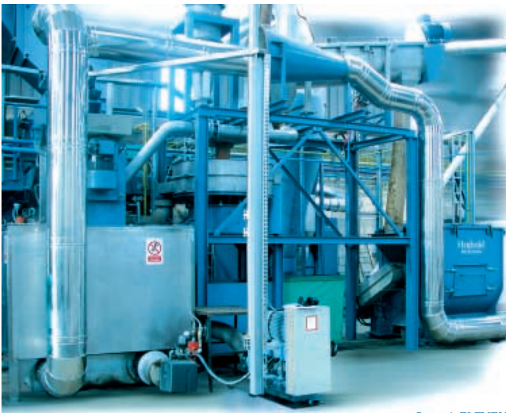
Hot washing plant for PET flakes
