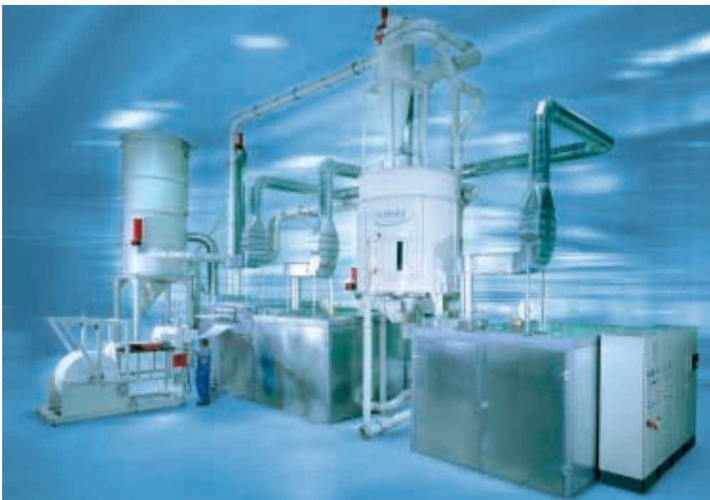
Pulverization plant for cellulose with three SMF 500/1000
