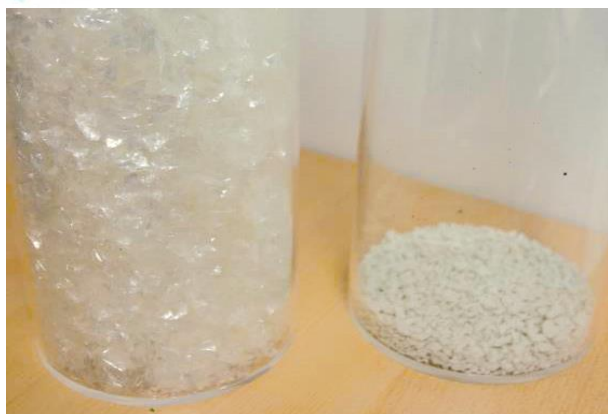
Picture shows 100g PET film as flake before processing and as agglomerate afterwards.
