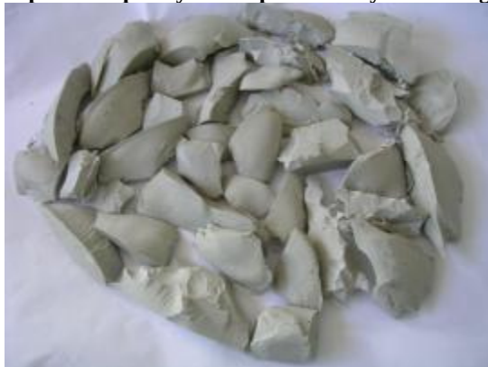
Typical granulate size after preliminary shredding approx. 50-100mm
