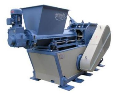
that, with rotor dimensions of 450 x 600 mm and a 37-kW drive, can attain a throughput of 1.000 – 1.200 kg/hr when grinding PET bottles (screen: 12 mm)
