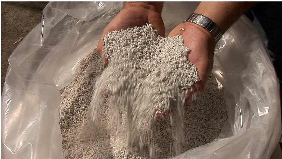
Fig. 1: The end product of the Herbold Plastcompactator is an agglomerate with high bulk density and excellent flow properties
