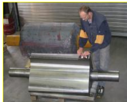
Fig.3: Blank and finished A rotor
