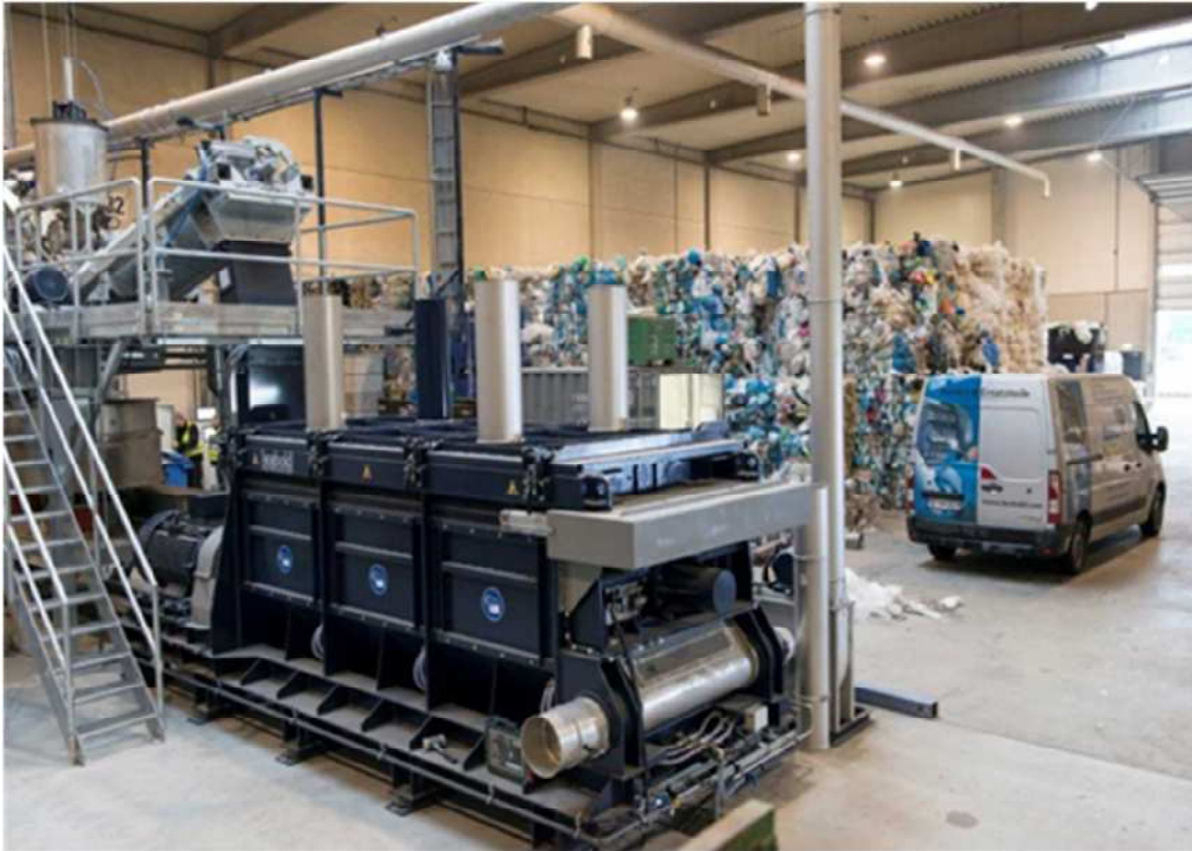
Fig. 3) Hydrocyclone and dryer, in the background pre-washing unit
