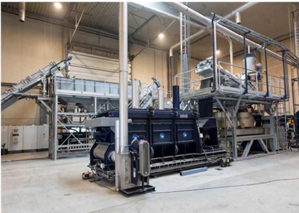
Fig. 3) Hydrocyclone and dryer, in the background pre-washing unit
